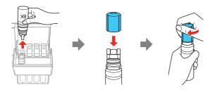
**Note:** Do not leave the ink bottle inserted; otherwise the bottle may be damaged or ink may leak. If any ink remains in the bottle, store the bottle upright for later use.
