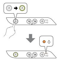
Press and hold the ♥ stop button for **5 seconds** until the ⊕ power light starts to blink and ink charging begins.
