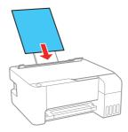
4 Slide the edge guides against the paper, but not too tightly, then flip the rear feeder guard back.
